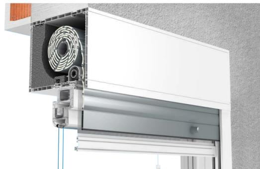
TP1000K shutter not built-up on both sides. For aesthetic purposes, the front profiles on both sides are smooth. The inspection cover in such a construction is from the bottom or from the front and the operation of the shutter is from the inside of the room.
