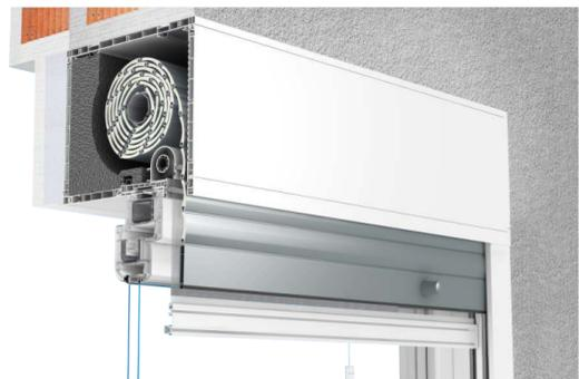
TP1000K shutter built-up from the inside. The internal front profile is grooved and equipped with a concealed lath. For better aesthetics, the external front profile is smooth. The inspection cover in such a construction is from the bottom and the operation of the shutter is from the inside of the room.
