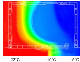
The top mounted roller shutters recommended most frequently by the manufacturers cause keeping the heat inside the building. In the layer between the shutter curtain and the window there is an airbag constituting an excellent insulating layer, i.e. a specific buffer, both for hot and cold air.
