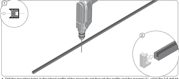
4. Drill the mounting holes in the lateral profile of the mosquito net through the profile and the magnet (1), using the 3.5 drill bit. The holes shall be drilled at every 50 cm and there shall be at least 3 holes in each profile. The bottom part of the profile shall be ended with the end cap (2).
