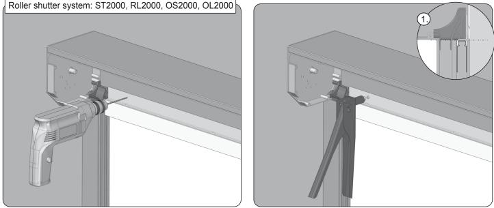
2. The so prepared upper rail of the mosquito net shall be fixed to the internal side of the roller shutter box. Make sure that the upper plane of the mosquito net rail is aligned with the upper end of the mosquito net guide (1). Using the 4.2 drill bit, drill the holes through the mounting angle bracket and the roller shutter box. The holes shall be drilled at every 50 cm and there shall be at least 3 holes in each profile.
