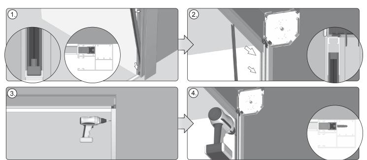
5. First, insert the lateral profile ended with the end cap in the groove of the mosquito net guide (1), next slide the profile towards the guide and make sure that the upper part of the lateral profile gets fitted into the upper profile (2). Screw the lateral profile, ended with the end cap, to the wall (3,4).
