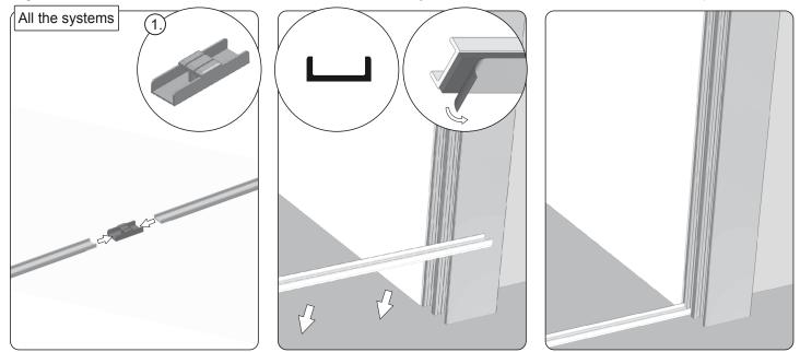
3. Connect the two bottom slats using the cord lock (1). The bottom slats shall be attached to the surface underneath by using the adhesive tape at the slat bottom.
