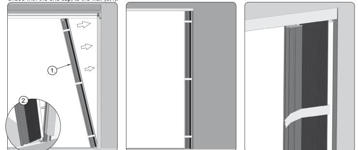
6. Start the installation of the mosquito net package from inserting the bottom part of the profile into the protruding mandrel of the bottom end cap on the lateral profile. Holding the package, remove the protection (paper tape) before unfolding the mosquito net.
