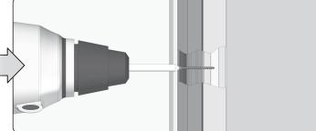
7. First, insert the lateral profile ended with the end cap in the bottom slat (1) by sliding the end cap into the slat, next slide the profile towards the mounting frame at the recess side and make sure that the upper part of the lateral profile gets fitted into the upper profile (2). Fix the lateral profile ended with the end cap to the guide of the blinds (3), using the 3,9x38 self-drilling screw.
