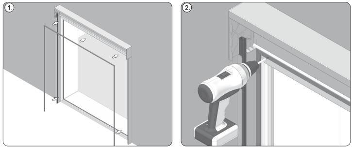
3. Fit the prior prepared mounting frame in the right installation position, between the guides, under the ZF3000-BX box (1). Fasten to the window frame (2) by inserting screws through the prior made holes and by tightening them.
