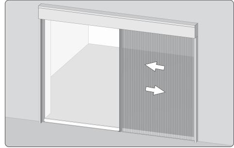
12. Check if the mosquito net works properly. If high resistance is felt during the sliding motion, decrease the tensioning of the cords, as presented in point 11. The second package of the mosquito net shall be installed on the opposite side following the same instructions as given for the first package, i.e. following the steps explained in points 8-11.
