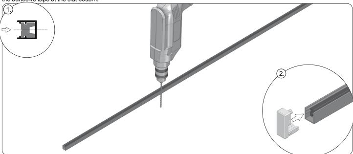
6. Drill the mounting holes in the lateral profile of the mosquito net through the profile and the magnet (1), using the 3.5 drill bit. The holes shall be drilled at every 50 cm and there shall be at least 3 holes in each profile. The bottom part of the profile shall be ended with the end cap (2).
