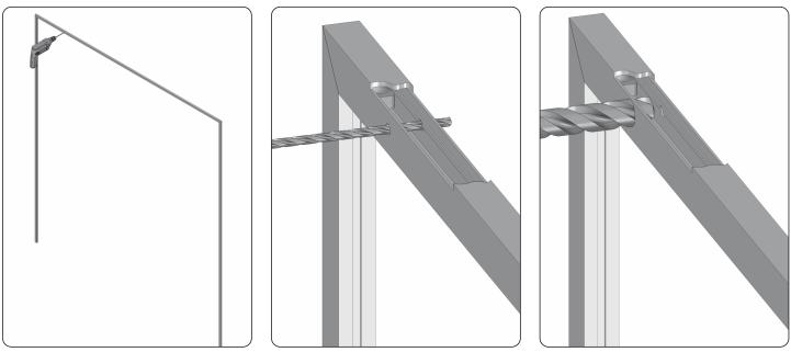
2. Drill the mounting holes every 50 cm in upper frontal profiles (at least 3 holes per profile): use the 4.2 mm drill bit, drill through both walls of the profile, next drill with the 7.5mm drill bit through 1 wall.
