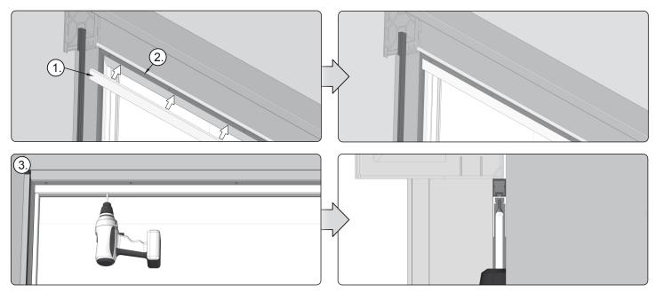
4. Lay the upper slat of the mosquito net (1) over the internal part of the upper profile of the mounting frame (2). Fix the slat to the frame (3) using screws.
