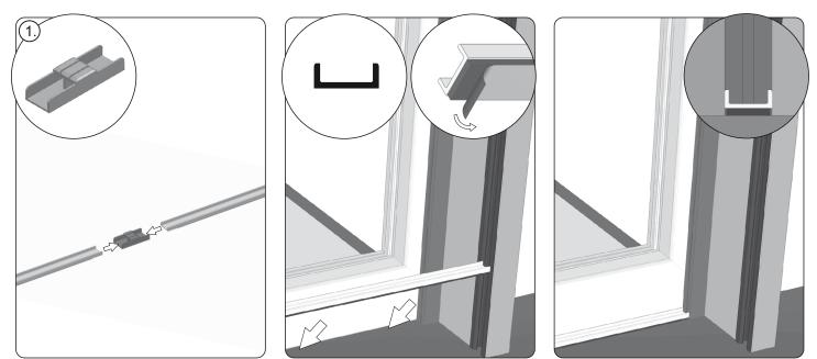
5. Connect the two bottom slats using the cord lock (1). The bottom slats shall be attached to the surface underneath by using the adhesive tape at the slat bottom.
