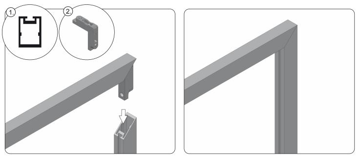
1. Assemble a mounting frame using frontal profiles (1) and connectors (2).
