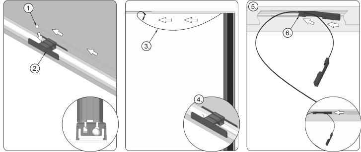
9. Stretch the bottom cords of the mosquito net. Make sure they do not get entangled, twisted or bundled. Put cord ends (1) in the cord lock of the bottom rail (2). Stretch the upper cord (3) so that the bottom cord gets properly tensioned and blocked (4). Properly place the upper cords. Pay particular attention and make sure that they are not entangled, twisted or bundled. As shown in figure 5, slide the element of the cord lock (6) through the milled hole in the upper rail in such a manner...
