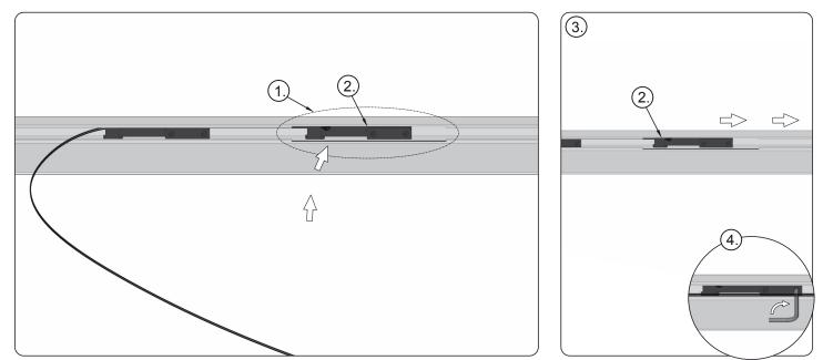
11. Insert the second lock (2) in the same milled hole (1) in the upper rail, slide the lock in the direction opposite to the first lock (3), this way, you will stretch the mosquito net cords. Fix the lock by tightening the socket head screws (4).
