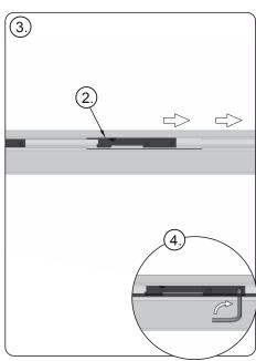
11. Insert the second lock (2) in the same milled hole (1) in the upper rail, slide the lock in the direction opposite to the first lock (3), this way, you will stretch the mosquito net cords. Fix the lock by tightening the socket head screws (4).
