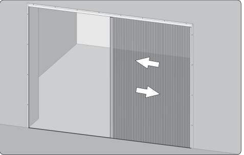
12. Check if the mosquito net works properly. If high resistance is felt during the sliding motion, decrease the tensioning of the cords, as presented in point 9. The second package of the mosquito net shall be installed on the opposite side following the same instructions as given for the first package, i.e. following the steps explained in points 4-9.
