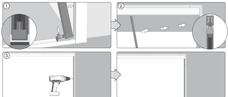
7. First, insert the lateral profile ended with the end cap in the bottom slat (1) by sliding the end cap into the slat, next slide the profile towards the mounting frame at the recess side and make sure that the upper part of the lateral profile gets fitted into the upper profile (2). Screw the lateral profile, ended with the end cap, to the wall (3).
