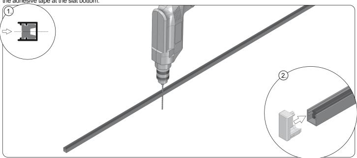
6. Drill the mounting holes in the lateral profile of the mosquito net through the profile and the magnet (1), using the 3.5 drill bit. The holes shall be drilled at every 50 cm and there shall be at least 3 holes in each profile. The bottom part of the profile shall be ended with the end cap (2).
