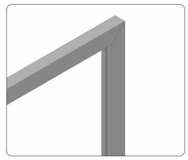
1. Assemble a mounting frame using frontal profiles (1) and connectors (2).
