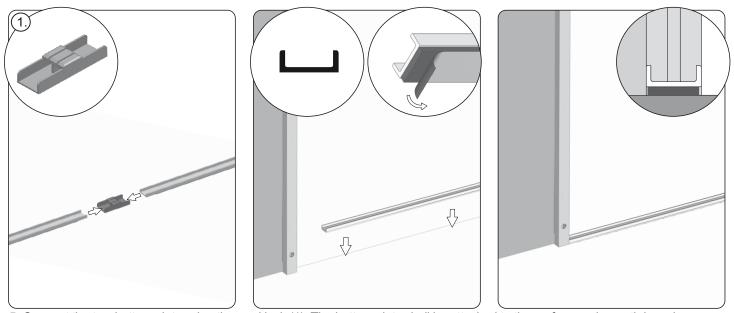
5. Connect the two bottom slats using the cord lock (1). The bottom slats shall be attached to the surface underneath by using the adhesive tape at the slat bottom.
