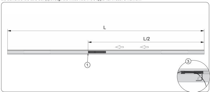
10. ...that the lock end (1) is exactly in the middle of the upper rail. Fix the lock by tightening the socket head screws (2).
