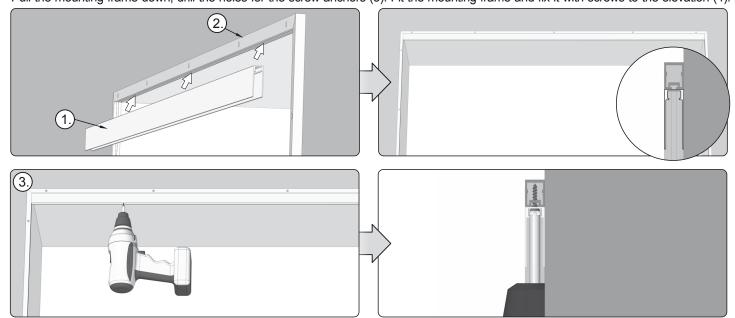
4. Lay the upper slat of the mosquito net (1) over the internal part of the upper profile of the mounting frame (2). Fix the slat to the frame (3) using screws.
