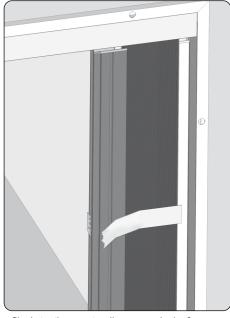
8. Start the installation of the mosquito net package from inserting the bottom part of the profile into the protruding mandrel of the bottom end cap on the lateral profile. Holding the package, remove the protection (paper tape) before unfolding the mosquito net.
