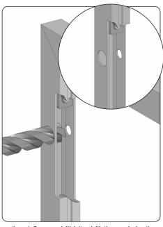
2. Drill the mounting holes every 50 cm in frontal profiles (at least 3 holes per profile): use the 4.2 mm drill bit, drill through both walls of the profile, next drill with the 7.5mm drill bit through 1 wall.
