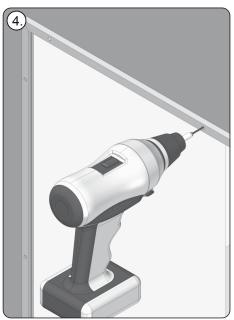
3. Fit the prior prepared frame in the right installation position on the elevation (1). On the wall, mark places for the mounting holes (2). Pull the mounting frame down, drill the holes for the screw anchors (3). Fit the mounting frame and fix it with screws to the elevation (4).
