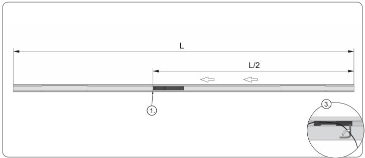
8. ...that the lock end (1) is exactly in the middle of the upper rail. Fix the lock by tightening the socket head screws (2).
