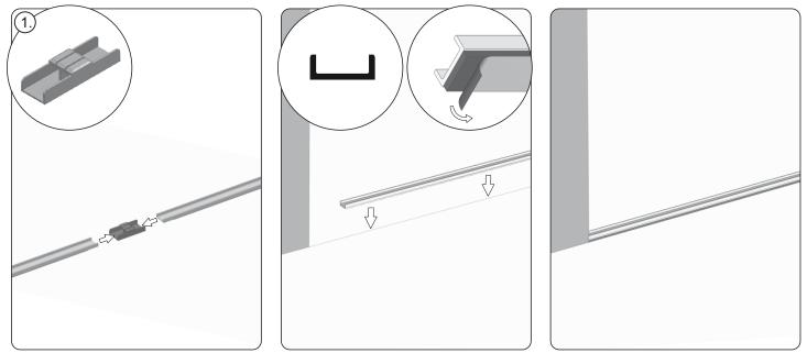
3. Connect the two bottom slats using the cord lock (1). The bottom slats shall be attached to the surface underneath by using the adhesive tape at the slat bottom.
