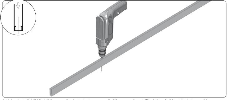
1. Using the 4.2 drill bit, drill the mounting holes in the upper rail of the mosquito net. The holes shall be drilled at every 50 cm and there shall be at least 3 holes in each profile.
