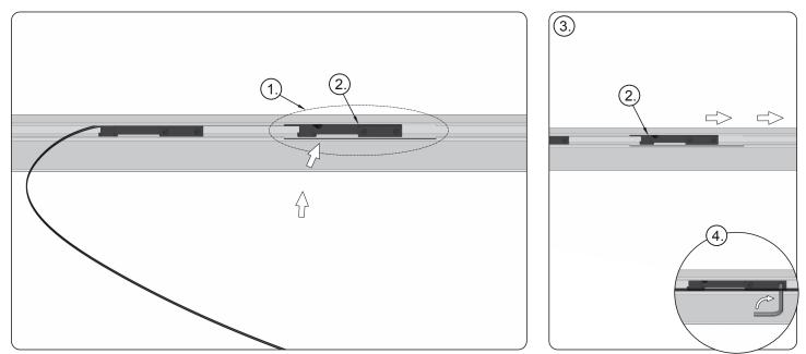
9. Insert the second lock (2) in the same milled hole (1) in the upper rail, slide the lock in the direction opposite to the first lock (3), this way, you will stretch the mosquito net cords. Fix the lock by tightening the socket head screws (4).
