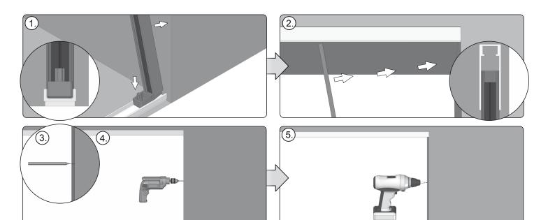
5. First, insert the lateral profile ended with the end cap in the bottom slat (1) by sliding the end cap into the slat, next slide the profile towards the mounting frame at the recess side, make sure that the upper part of the lateral profile gets fitted into the upper profile (2). On the wall, mark position of the holes (3), remove the lateral profile. Next, drill holes for the screw anchors (4). Screw the lateral profile, ended with the end cap, to the wall (5).
