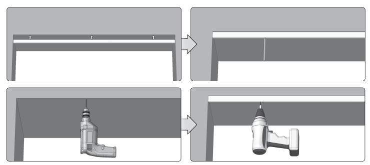
2. Fit the upper slat of the mosquito net in the upper recess of the door opening, mark and drill holes for the screw anchors.
