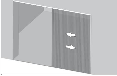
10. Check if the mosquito net works properly. If high resistance is felt during the sliding motion, decrease the tensioning of the cords, as presented in point 9. The second package of the mosquito net shall be installed on the opposite side following the same instructions as given for the first package, i.e. following the steps explained in points 4-9.
