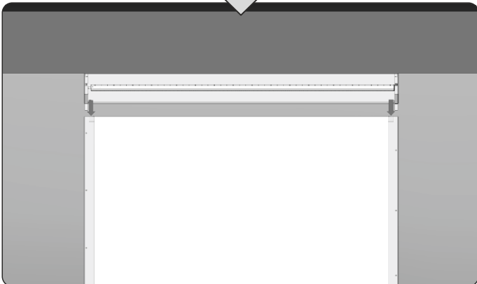
11. Slide the box onto the screwed guides.
