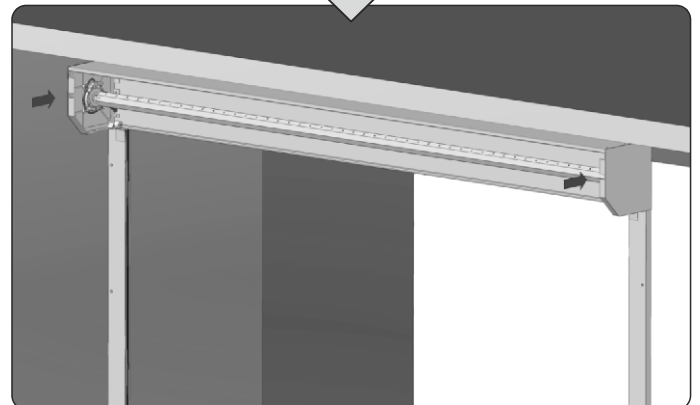
11a. Insert the complete set into the recess.
